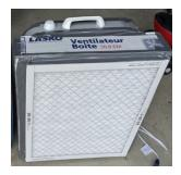
When there's no space for a four-filter box, a one-filter version is useful. It's less expensive to make, although the filter needs to be changed more often.
