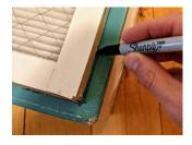
With the box the right way up, centre the filter on it. Pleats should be vertical. Trace around the edges.
