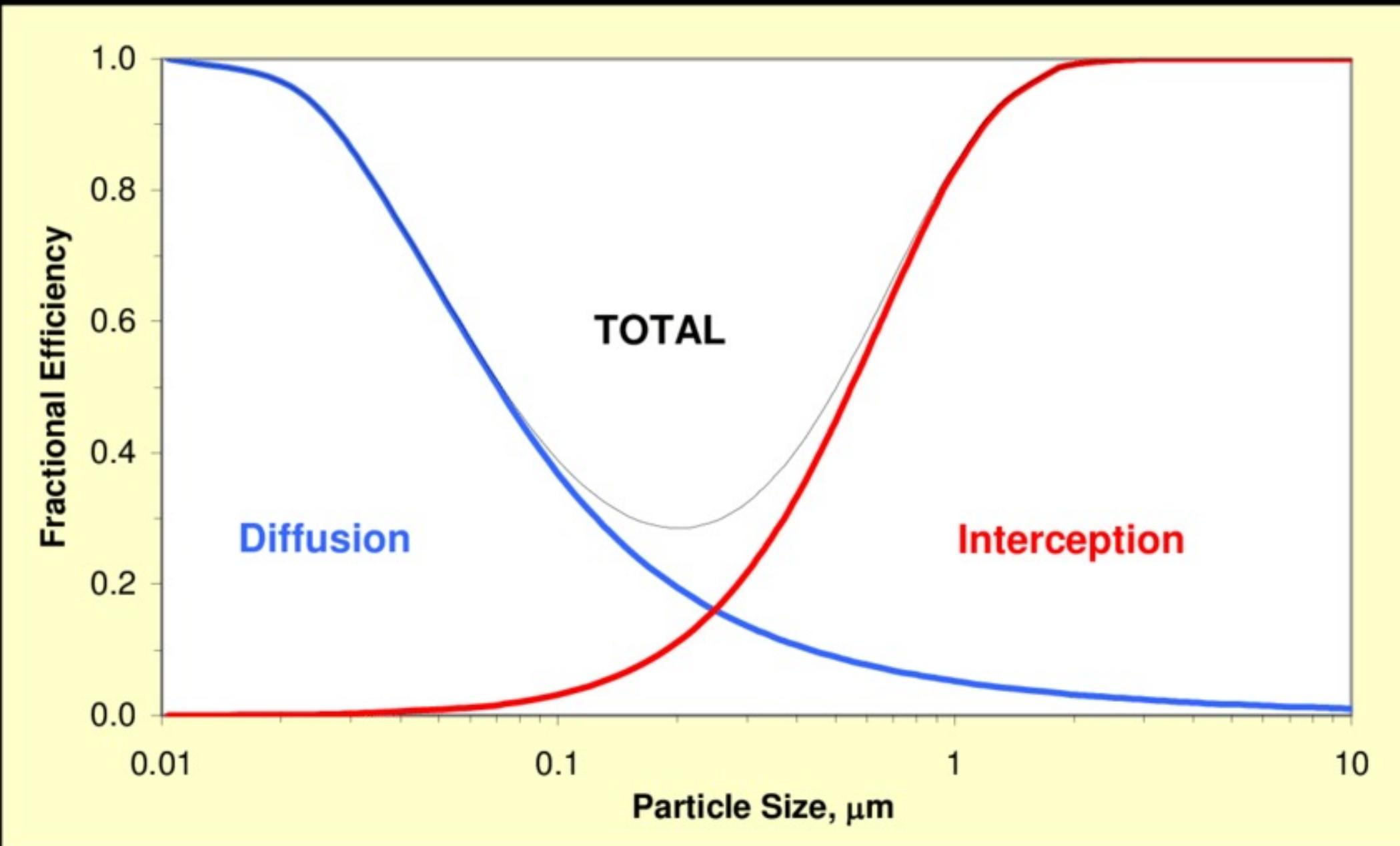
Generalized performance curve for a filter showing components.
