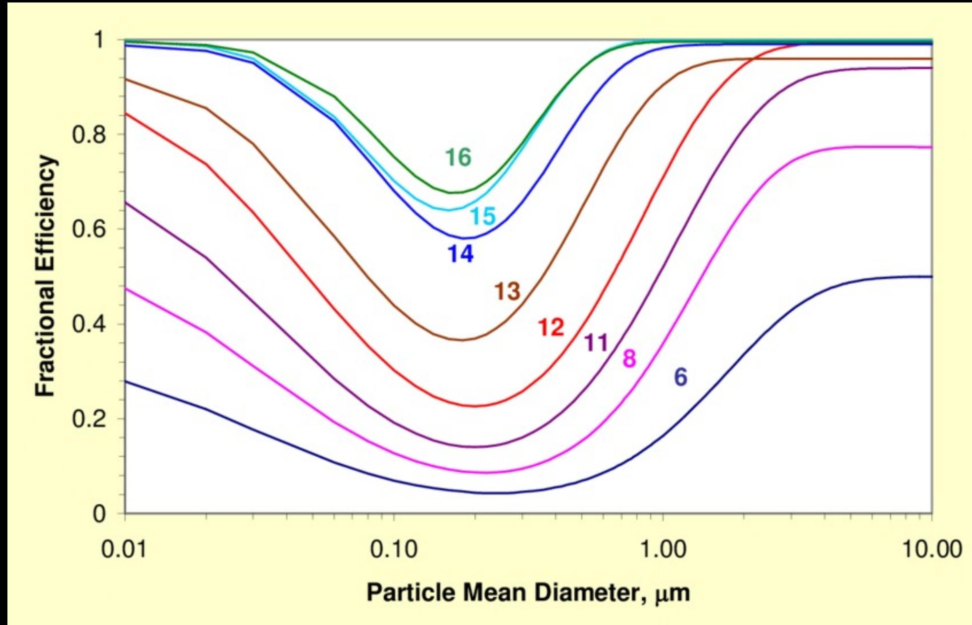
Composite of all MERV filter models, based on initial conditions.
