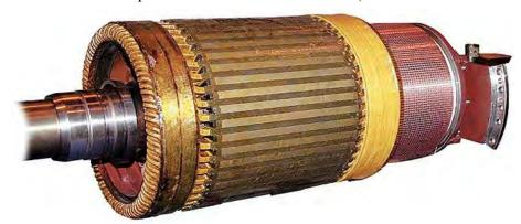
the coils. The wedges were plastic in nature and called Epon glass wedges. (Like a plastic divider)
