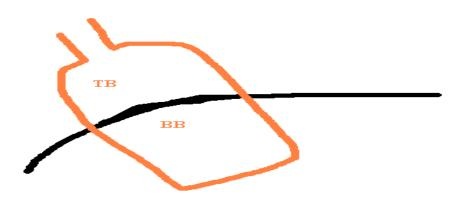
FORMING AND BENDING: PART IS CLAMPED DOWN WITH A STEEL STRAP. THE BOTTOM BARS ARE LAID DOWN WITH GLASTIC. 'THE REST OF THE PROCESS INVOLVED INTRICATE STEPS OF LINING AREA WITH MICA MAT AND WEDGING WITH TEXTOLITE WEDGES.
