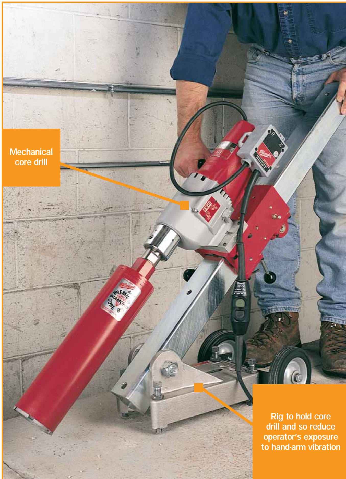
Figure 8. Example of using a rig to operate a power tool
