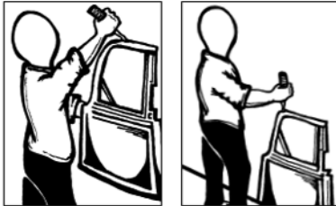
Figure 3: Working with the arms above shoulder height increases the risk of developing shoulder injuries. Awkward postures can be reduced by raising the worker on a platform and/or lowering the work piece.
